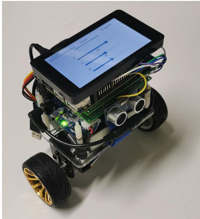
Figure 1.1: Self-balancing robot controlled by the STM32MP1
