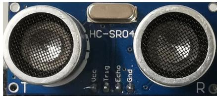
Figure 5.34: Ultrasonic sensor
