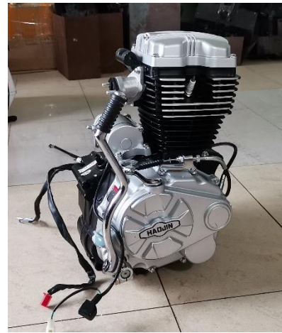
ICE fuel motorbike engine removed from the motorbike
