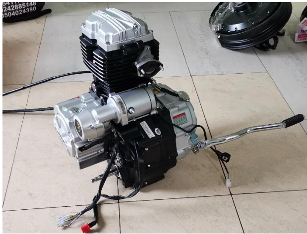
ICE fuel motorbike engine removed from the motorbike
