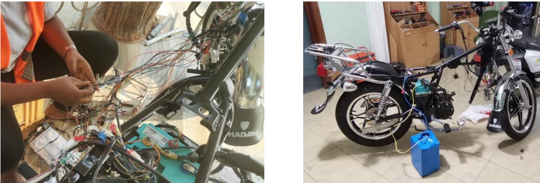
Electrical rewiring of the ICE fuel motorbike
