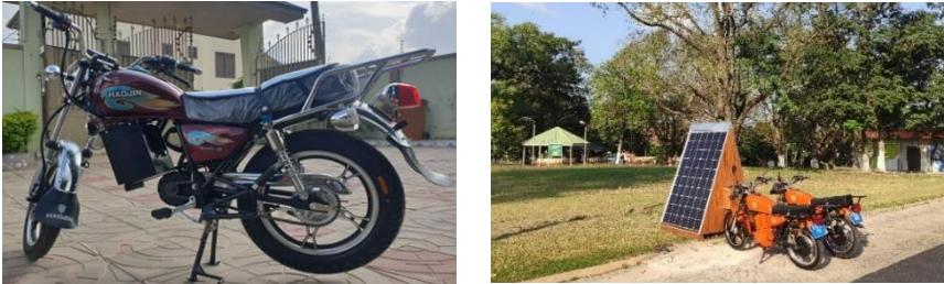
**Fig.2a.** Conventional motorbike stripped internal combustion engine (top right, Model: Haojin 125-32, 150cc)
