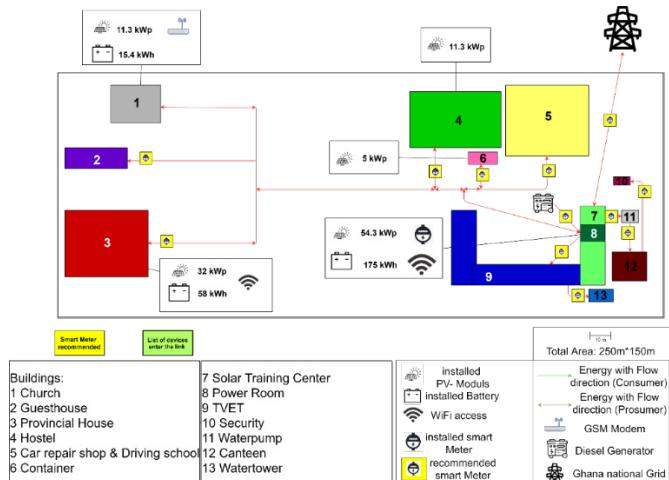
Fig. 2: Sketch of the Don Bosco Mini Grid
