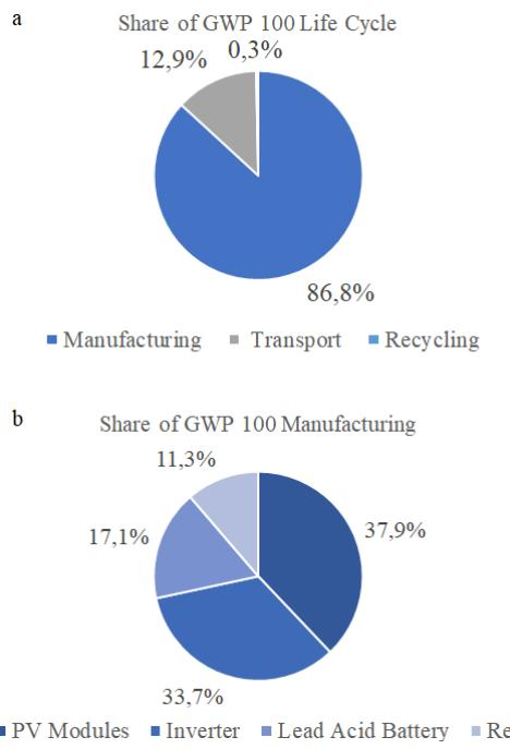
Fig. 3. (a) total amount of GWP emissions; (b) share of GWP for the Don Bosco Mini Grid
