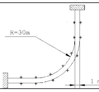
Figure 6: 'Figure-8' track test
