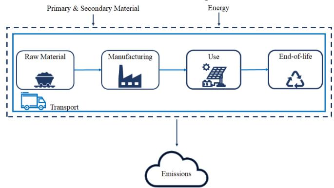
Fig.1. system boundary diagram for the life cycle assessment of the Mini Grid
