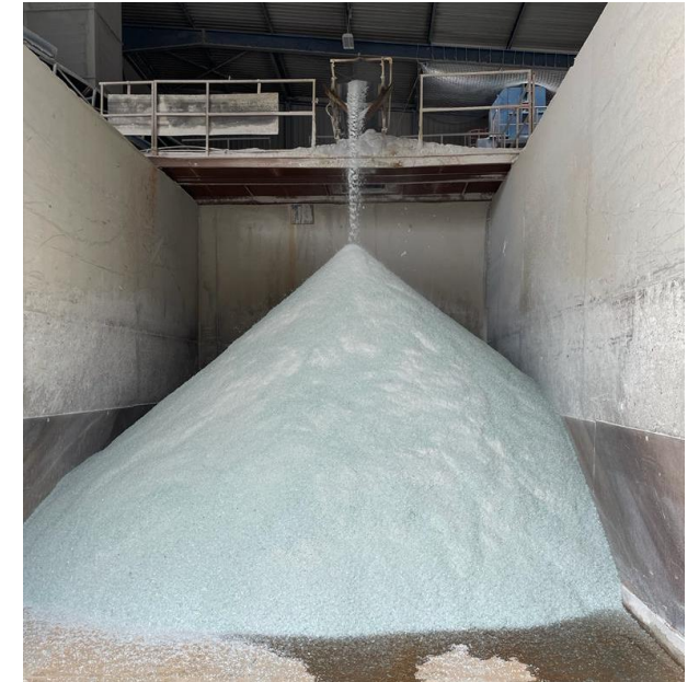
Recycled glass of PV panels
