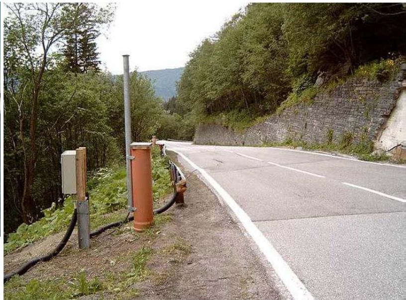
Fig. 4 (right): GPS-point for monitoring the slope close to a road
