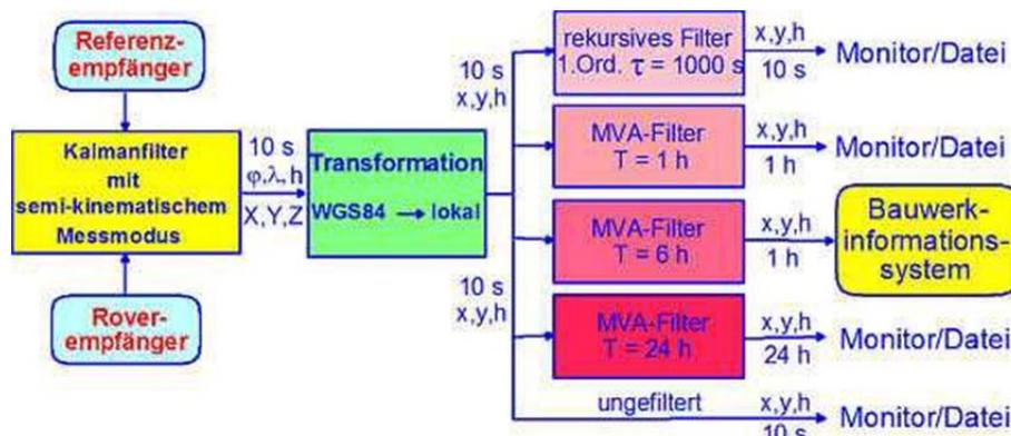
Fig. 5: Overview of the algorithms of the SMMS
