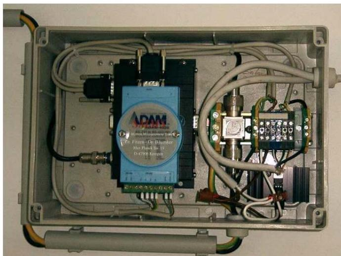
Fig. 1: 8-channel GPS-receiver with RS422/232-converter and lightning fuse
