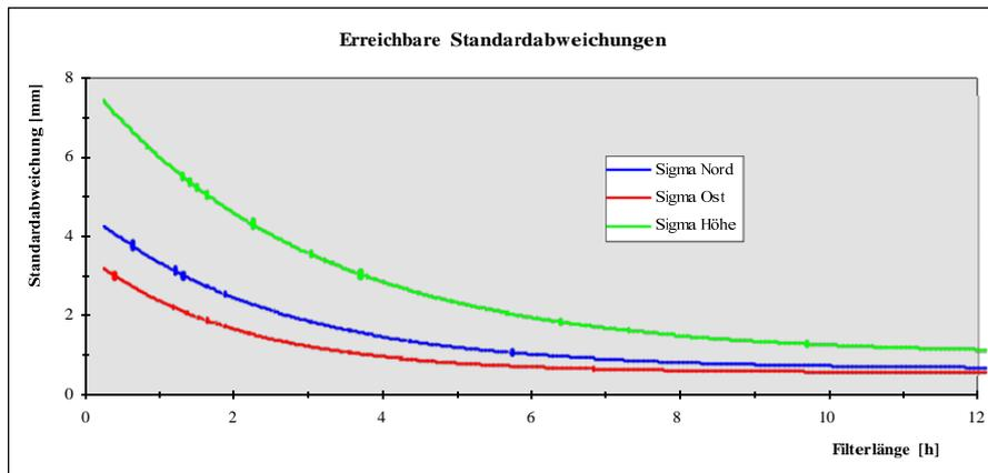
Fig. 6: Typical standard deviations (north, east, height) (95%) in dependency of the filter length
