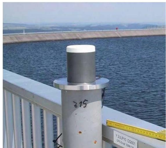
Abb. 2: GPS-antenna with mounting
